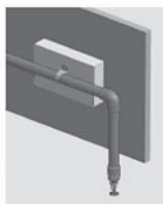
Branches Supported with Blocking
