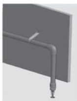
Branches Supported with Hangers
